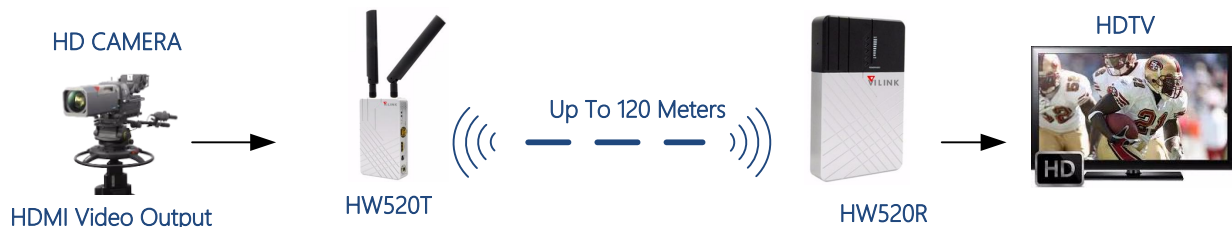
Typical HW520T & HW520R Application
