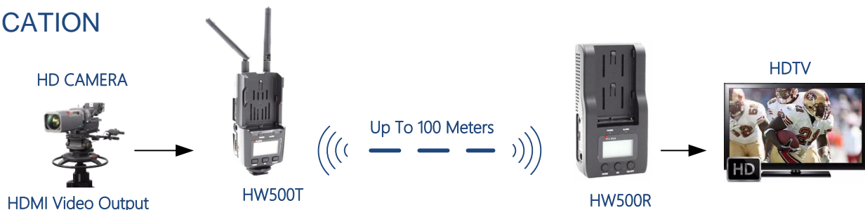
Typical HW500T & HW500R Application
