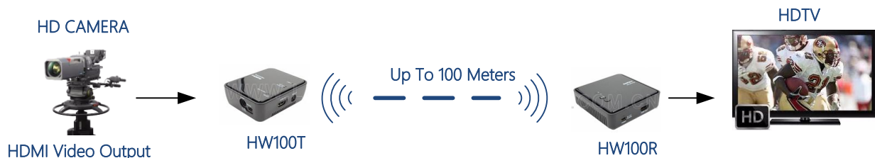
Typical HW100T & HW100R Application
