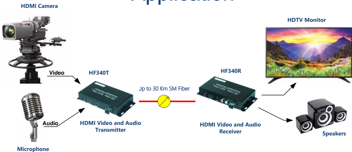
Typical HF340T & HF340R Application
